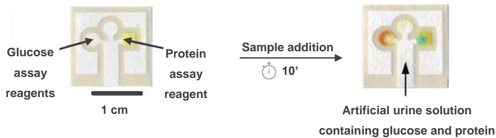
Figure 4. Paper-based analytical device created by Whiteside's group. A) Glucose is tested in the circular region on the left, while protein is tested on the square region on the right. The circular region on the top was used as a control. B) After addition on the central channel, the sample is guided to the three reactive chambers by capillary action. Positive results for glucose and protein are presented on the left and on the right, respectively. Adapted from [20]
