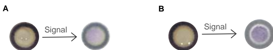
Figure 15. Polyvinyl alcohol and Triton X-100 effect on the signal obtain. A) When no surfactants are added, sample drops do not spread easily through the surface, affecting signal homogeneity. B) In the presence of surfactants, spot surface became more hydrophilic, so drop spreading was facilitated and a higher signal homogeneity was achieved.
