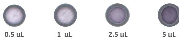
Figure 17. Evaluation of the minimum volume required to obtain an adequate visual read-out. Different volumes of mix were spotted and dried. Tests were made with a solution of 600 mg/L of L-malic acid supplemented with \text{NAD}^+ and Tris plus glutamate.
